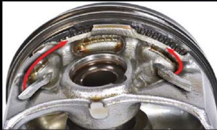
Example of piston damage due to an LSPI event observed during the testing of a competitor's motor oil. The red arrows indicate sections of the ring land that broke away from the piston.
